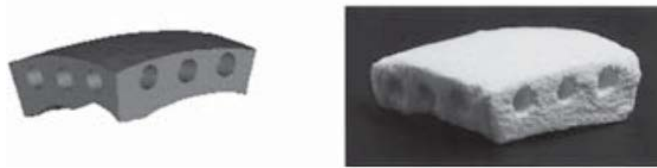
Figure 2.12: Implant design model fabricated using CAD and the tailor-made bone implant after ink-jet printing.
