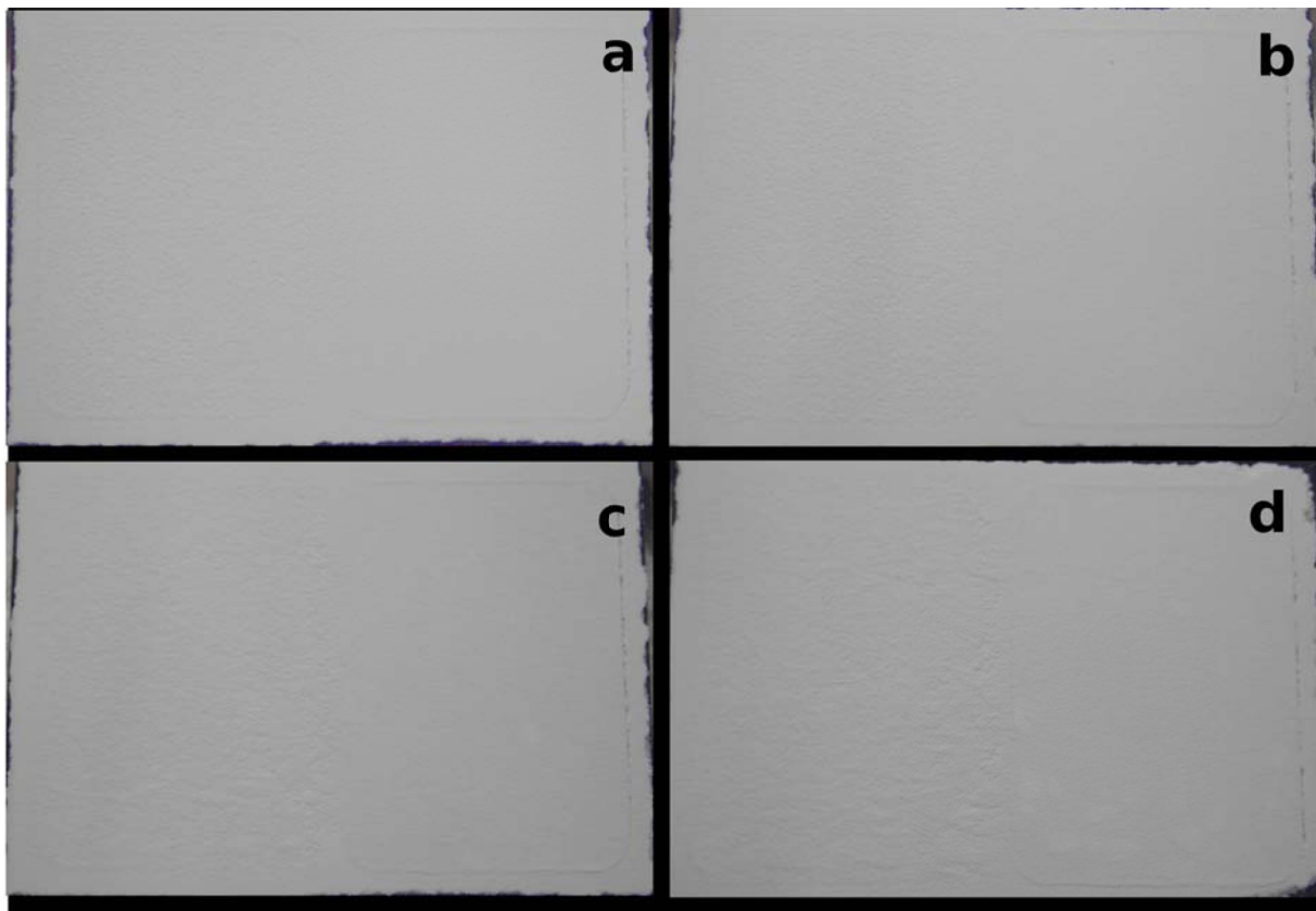
Figure 4.11: Powder bed deposition of the coarse \alpha -TCP powder after 15 layers with gas flow. a) 5-50-2.5-105, b) 10-50-2.5-105, c) 50-50-2.5-105, d) 70-50-2.5-105. The left side of the powder bed is the build bed while the right side is the feed bed.
