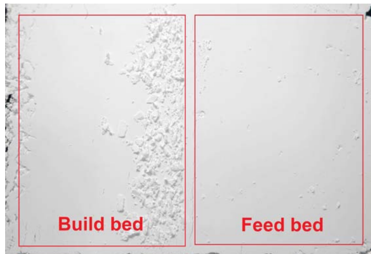
Figure 4.9: Powder bed deposition of the fine \alpha -TCP powder without brush. The left side of the powder bed is the build bed while the right side is the feed bed.
