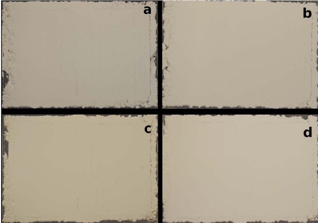
Figure 4.13: Powder bed deposition of the fine \alpha -TCP powder after 15 layers with gas flow. a) 10-10-3-120, b) 10-10-3-80, c) 20-10-3-50, d) 40-10-3-30. The left side of the powder bed is the build bed while the right side is the feed bed.
