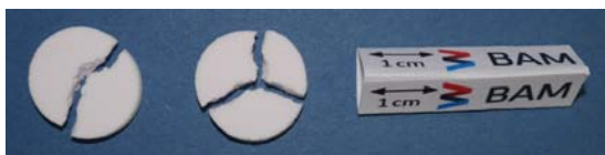
(a) Coarse powder tablets printed without gas flow.
