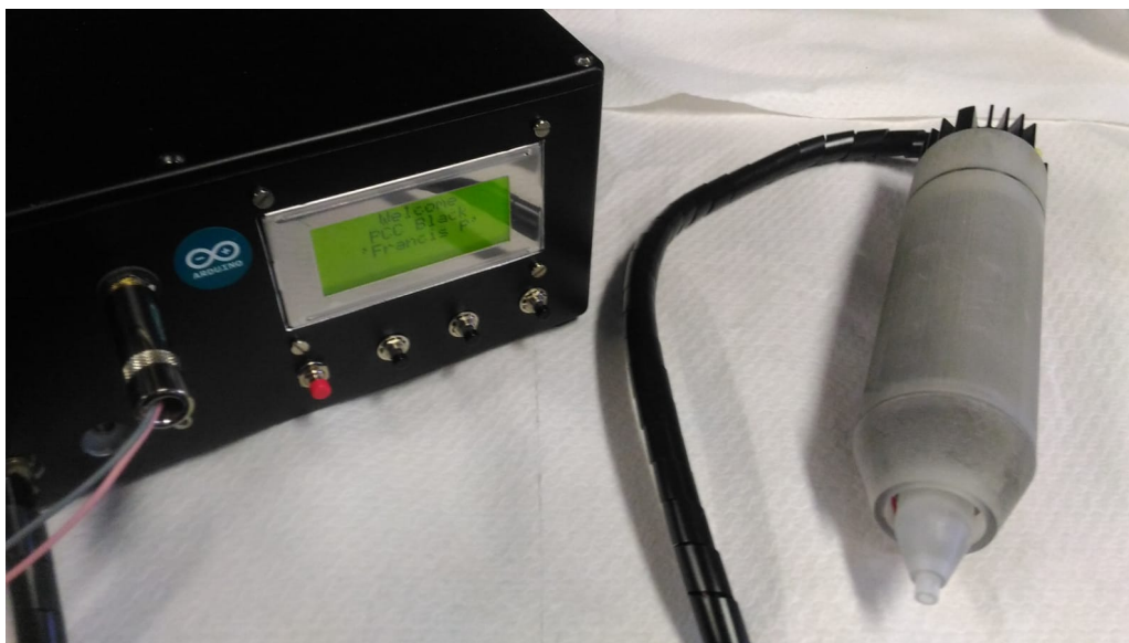
Figure 2.2: Picture of PCC source, prototype B . The black box on the left is the Controller , the cylinder on the right is the Head where plasma is produced.
