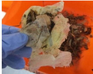
Figure 4.23-Bioplastic lumps formed during the composting process
