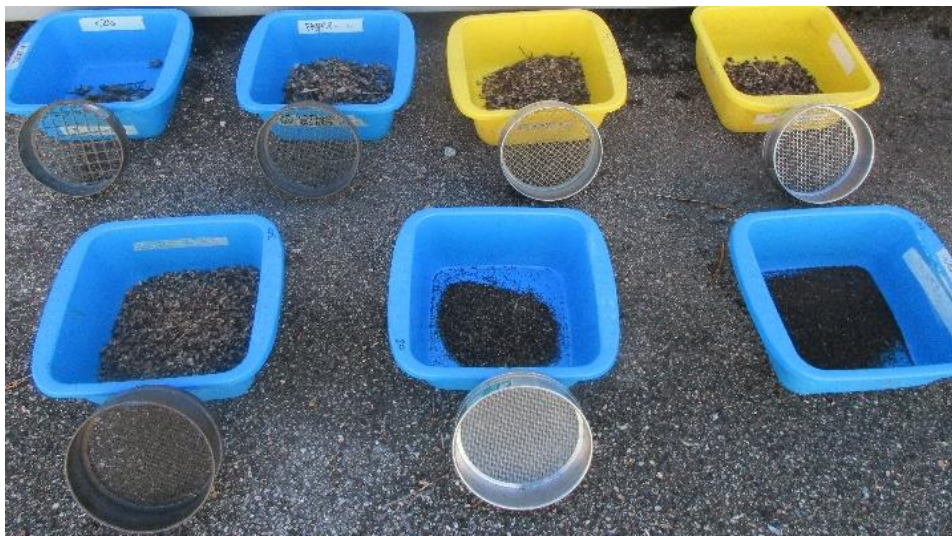
Figure 4.11-Sieved fractions 10th day, OF (F. Ruggero, 2017)
