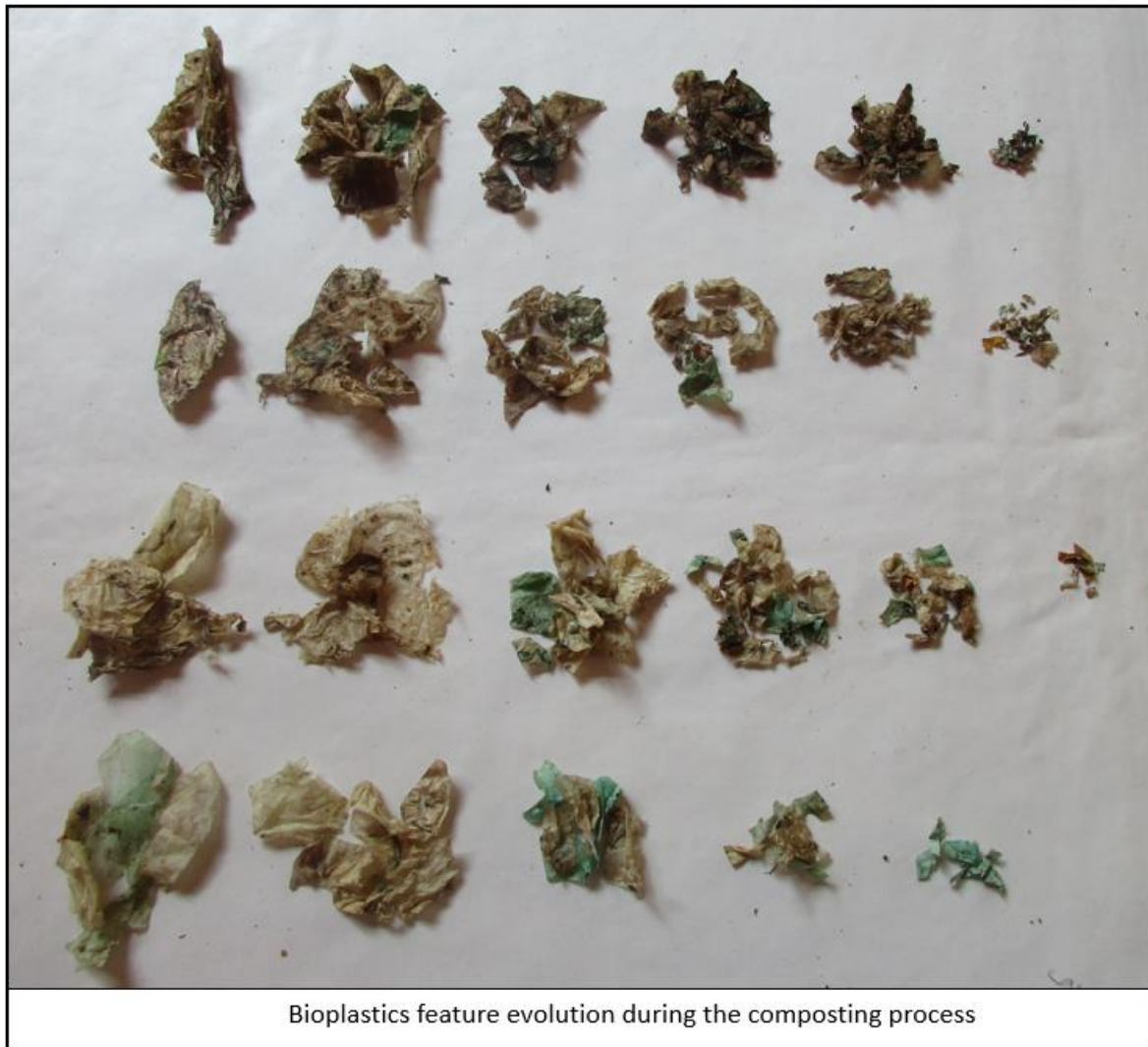
Figure IV.1-Aspect of bioplastic pieces submitted to IR analysis
