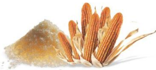
Figure 2.13-Mater-Bi in granular form. They are made on corn-starch and biodegradable polyesters (www.novamont.com)
