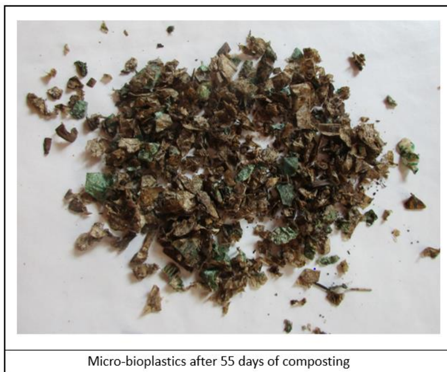
Figure 4.35-MicroBioP aspect after 55 days (F. Ruggero, 2017)
