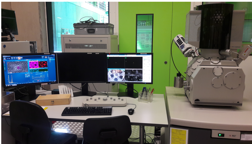
Figure 5.3: FEI Verios460 XHR SEM employed in this work. Since it is provided with a X-ray detector, also the EDX analysis has been performed with this instrument.
