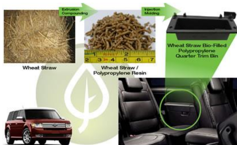
Figure 2.5 Application of natural fibres in a car
