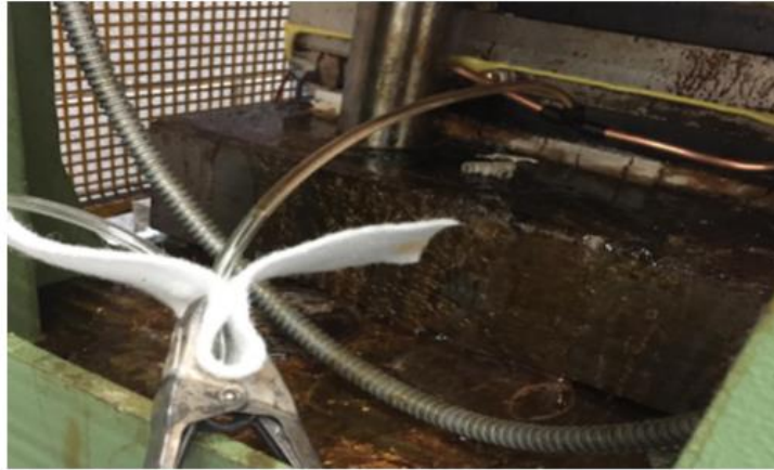
Figure 5.18 Resin extrusion in the vacuum tube
