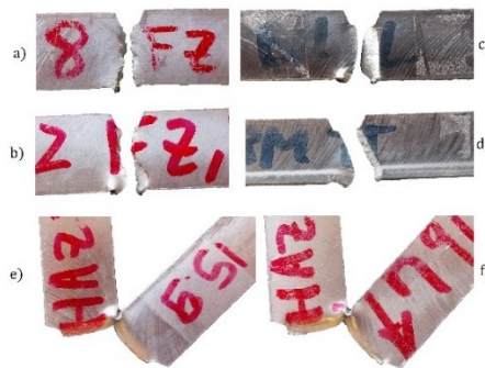
Figure 4.25: Macro images of the Charpy V-notch specimens after testing.
