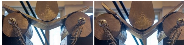
Figure 4.5: Bending of the parent material.
