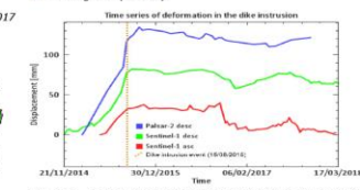
Figure 11. Time series of deformation in the dike intrusion, obtain from Palsar-2 descending data (blue line), Sentinel-1 descending data (green line) and Sentinel-1 Ascending data (red line). The orange dashed line highlight the time when the dike intrusion occurred (15 August 2015)
