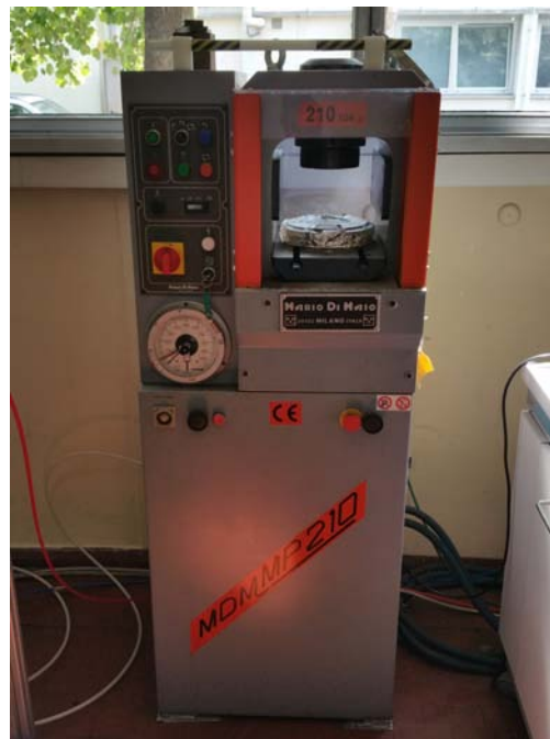
(c) Automatic hydraulic press.
