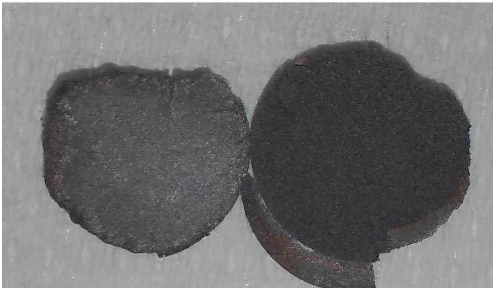
(b) Difference between the two sample sides. The right one was in contact with graphite plate, while the other one was free.
