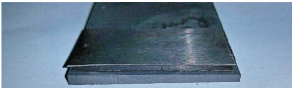
Figure 5.22: Samples were placed between two tantalum sheets to prevent Ge evaporation.
