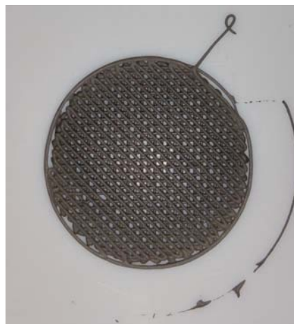
(b) The 45^\circ green maintain its shape just after printing.
