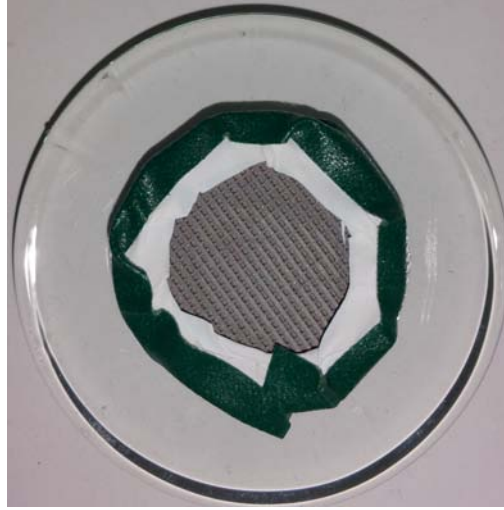
Figure 6.20: TiC 3D sample preparation for a permeability measurement.
