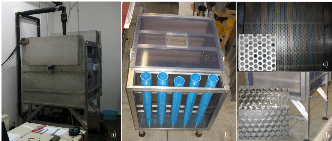
Figure 2.2: a) The experimental apparatus in test configuration. The insulated circuit of the copper heat exchanger is visible; b) A view from the top of the filtration fluid inlet tank with the micro-pitted pipes; c) The perforated stainless steel wall; d) A detail of the flow rectifier located between the micro-pitted pipes and the perforated wall.
