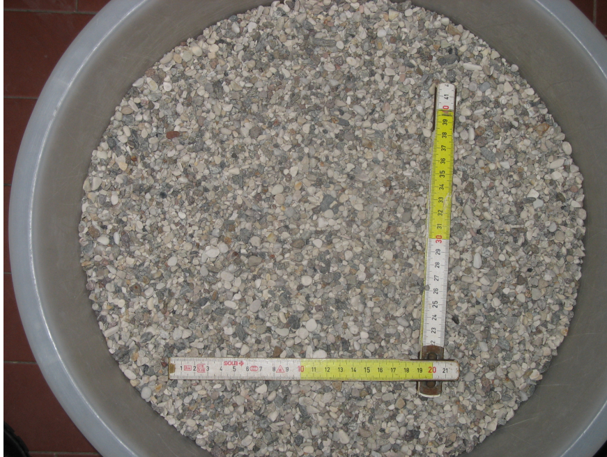
Figure 3.1: Risetta del Brenta , the granular material adopted in the test.
