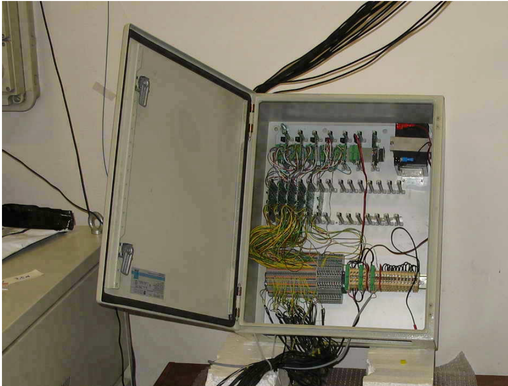
Figure 3.3: The acquisition system endowed with 42 channels for the acquisition of data from the experimental apparatus.
