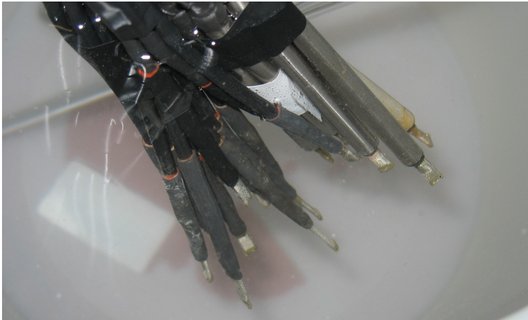
Figure 2.6: PT100 Resistance Temperature Detector with the metal sock protection used in the test.
