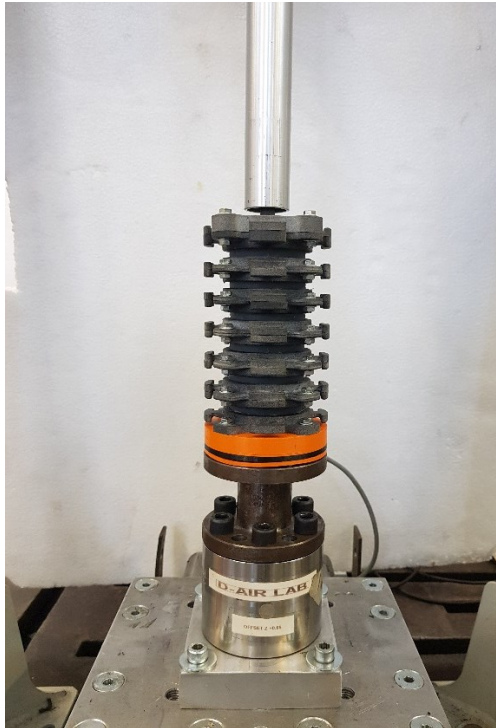
Figure 4.16: Setup for the axial compression test
