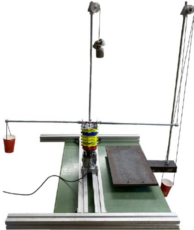
Figure 4.1: Static test bench for bending stiffness evaluation employed by Rango M [32].
