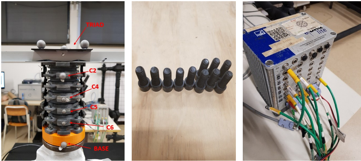
Figure 4.3: From the left to the right, markers configuration on the neck, samples of screws used as weights, Data Acquisition System
