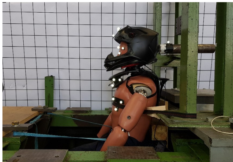
Figure 6.12: Improved test setup for back impact
