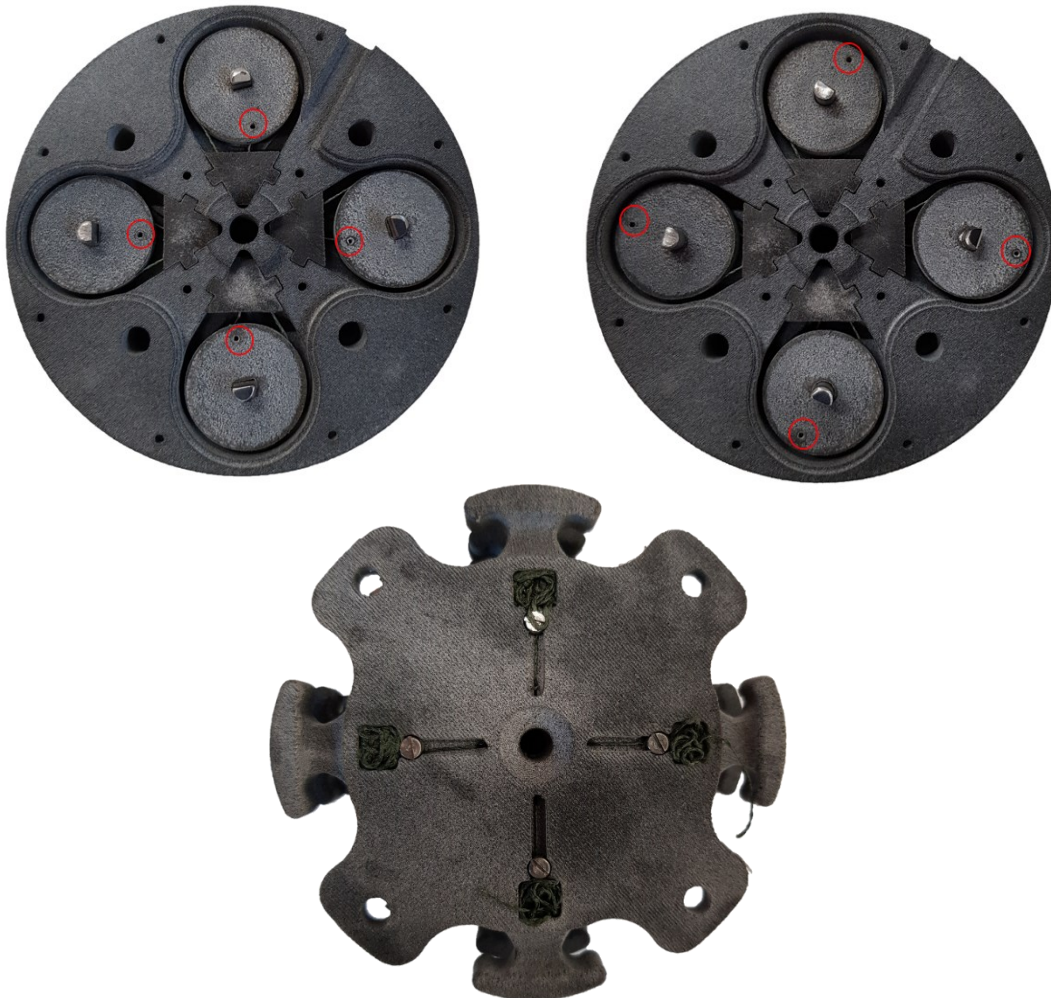
Figure 5.14: On the top unloaded and loaded configuration of the instrumented base, on the bottom the upper vertebra where the four cables are fixed by winding them around the screws
