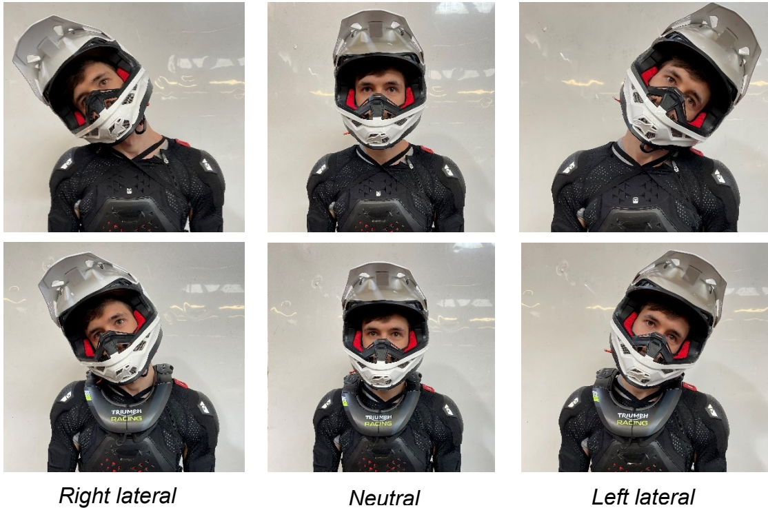
Figure 6.1: On the top the ROM of the head in lateral bending without neck brace, on the bottom the ROM of the head in lateral bending with neck brace
