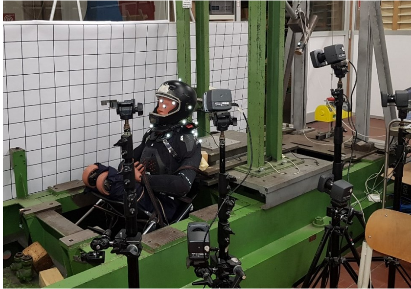
Figure 6.4: Impact test setup
