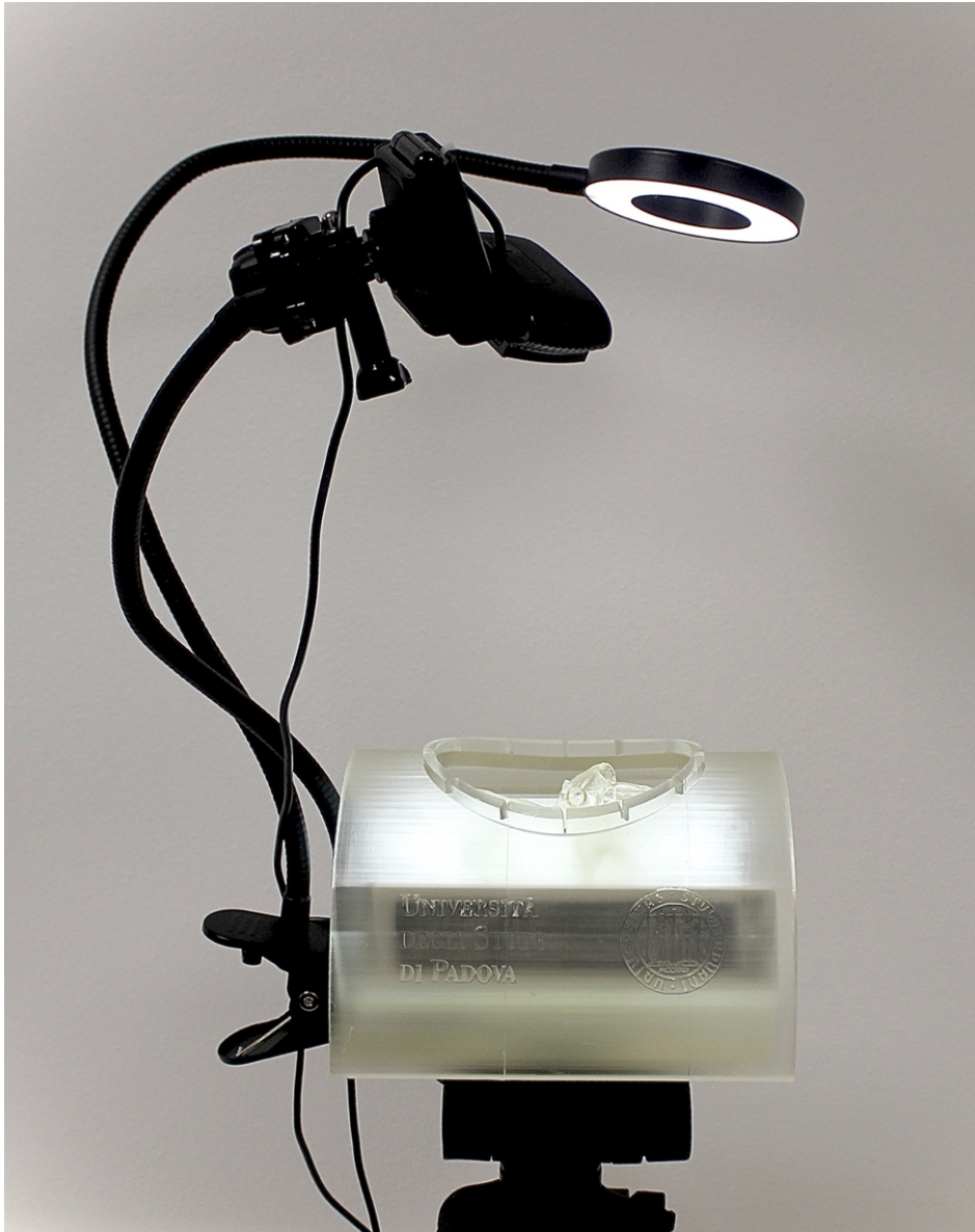
Figure 41 - Congenital TrainHeart attached to the tripod with the external light and webcam allowing surgical procedure to be recorded or live supervised by a tutor.
