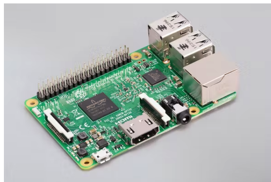
Figure 3.5: Raspberry Pi 3 Model B - A single-board computer with wireless LAN and Bluetooth connectivity
