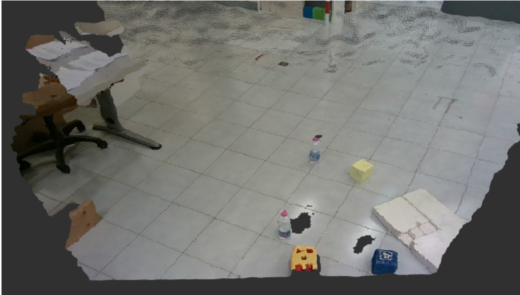
Figure 2.2 An example of input Point Cloud visualized in RViz
