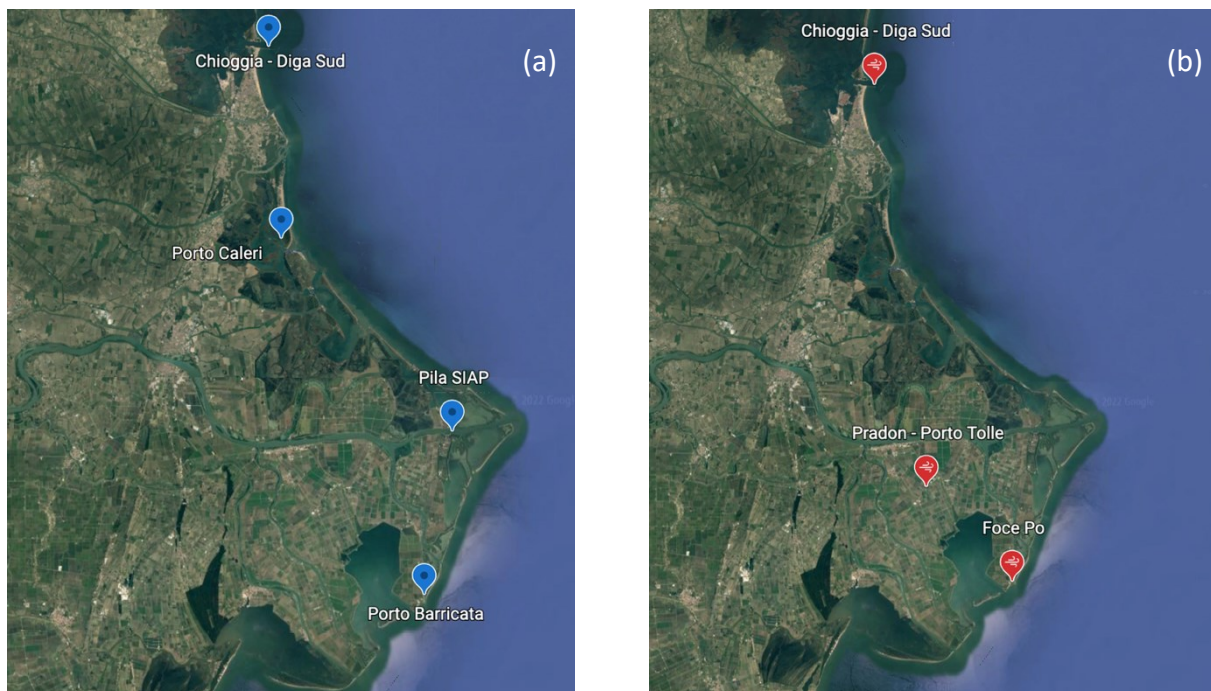
Figure 3.2: Location of level (a) and wind (b) measurement stations.
