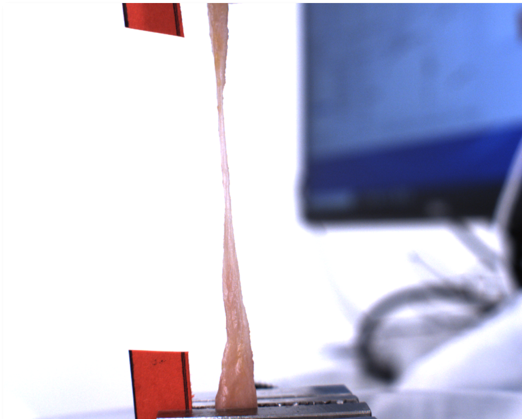
Figure 3: A Fascia lata specimen after the uniaxial tensile test
