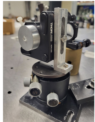
Figure 2.6: Pictures of the second crystal holder, with the crystal inserted in it, mounted on the vertical stage, on the rotating platform.
