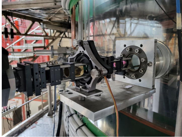
Figure 4.29: Picture of the second half of the DI on PROTO-SPHERA, mounted on the machine.
