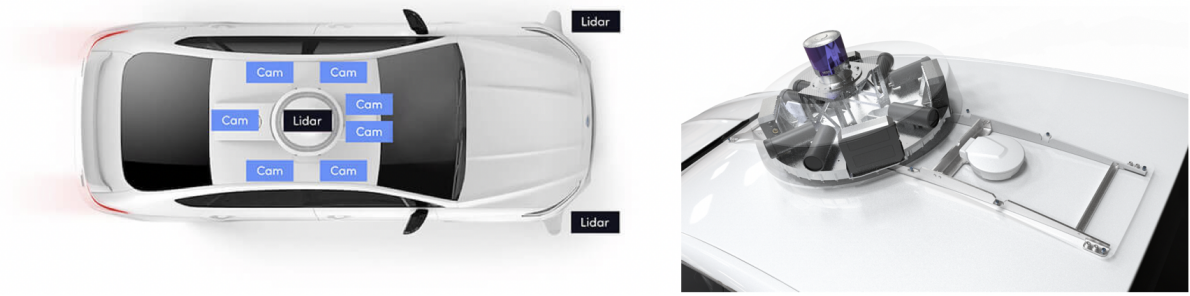
Figure 2.6: Level 5 Automated Vehicle sensors
