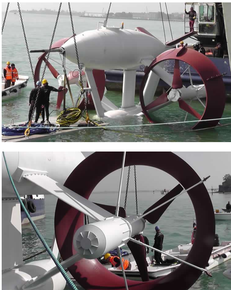
Figura 17: Full-scale photo of the prototype in the Venice lagoon and detail of the turbine (from SEAPOWER)
