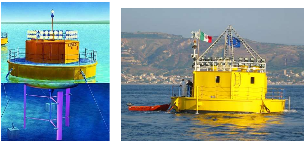
Figure 11: Schematic representation and photo of the Kobold TEC
