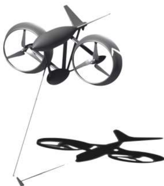
Figure 15: CAD Representation of GEMSTAR Single Cable Anchor (from SEAPOWER)
