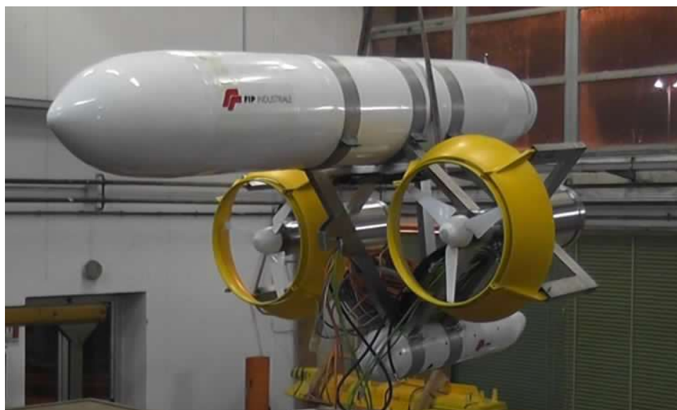
Figure 16: Photo of the second 1:5 scale prototype of the GEMSTAR model
