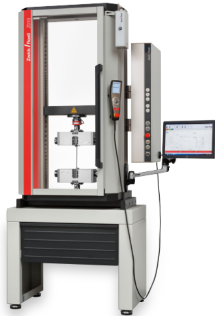
(b) ZwickRoell AllroundLine universal static tester.
