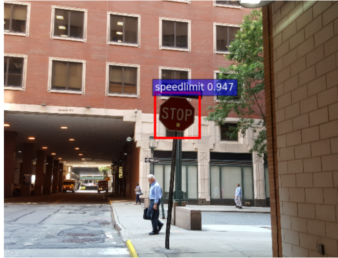
Figure 1.1: Example of a backdoored street sign classifier. The stop sign is maliciously misclassified as a speed-limit sign by the malicious model [10].
