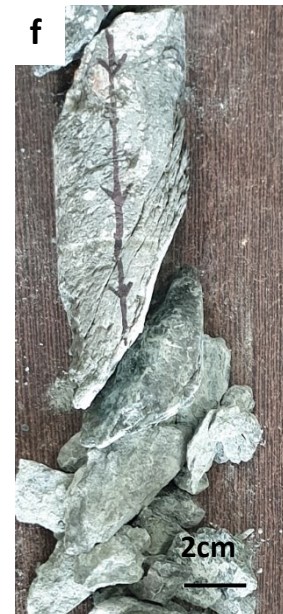
Figure 3.5f. Fractured and altered foliated shear zone from KBH6 (photo by Di Toro, 2019, Karad repository)
