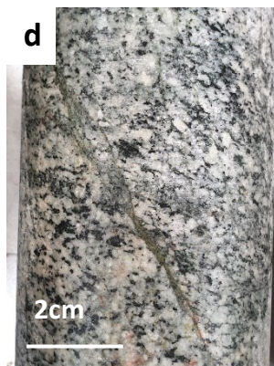
Figure 3.5d. Granitoid, possibly a tonalite, KFD1, cut by a steeply-dipping epidote-bearing fault (photo by Di Toro, 2019, Karad repository).
