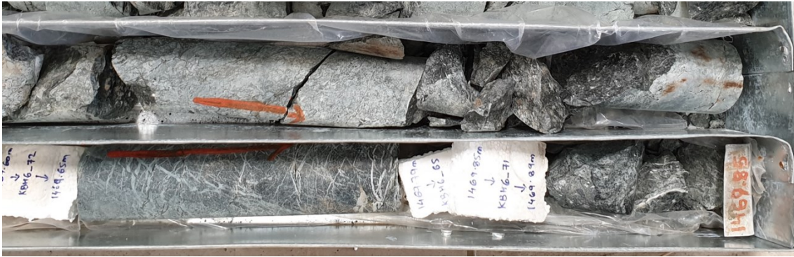
Figure 5.7. Core sample from Karad repository with the dense network of quartz sealed by quartz veins.
