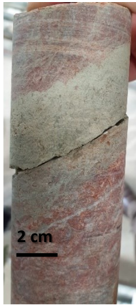
Figure 5.5. Sample KBH1-352 showing a fault/fracture filled by epidote vein cutting through the granite basement.
