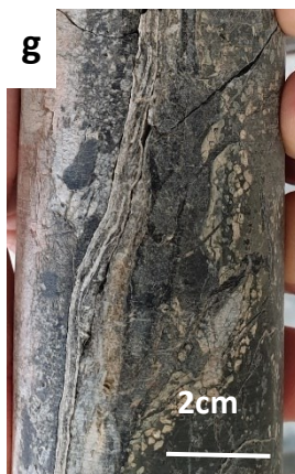
Figure 3.5d. Granitoid, possibly a tonalite, KFD1, cut by a steeply-dipping epidote-bearing fault (photo by Di Toro, 2019, Karad repository).
