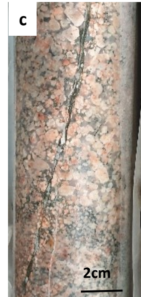
Figure 3.5c. Granite cut by a steeply-dipping fault filled first by chlorite and then by later calcite veins (photo by Di Toro, 2019, Karad repository).
