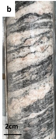
Figure 3.5b. Proterozoic Migmatitic gneiss from KFD1 with alternation of leucosomes (white bands) and melanosomes (black bands) (photo by Di Toro, 2019, Karad repository).
