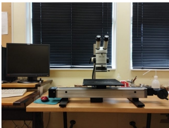
Figure 16. Rinntech LINTAB measuring apparatus (on the left) at the dendro lab of the Icelandic Forest Research (division of the Icelandic Forest Service (Skógræktin)), in Mógilsá, Reykjavík; some of the birch core samples (on the right) glued on wooden supports.
