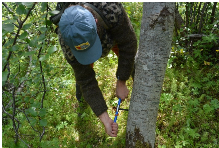
Figure 15. Coring of a tree with an increment borer. Pagnan, G. summer 2022.
