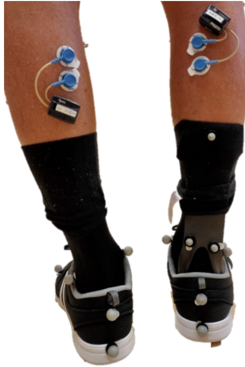
Figure 37: A custom AFO (on the right leg) with the three markers placed on the posterior calf shell (one on the upper extremity, the other two on the lower one along the ankle bending axis passing through the malleoli).
