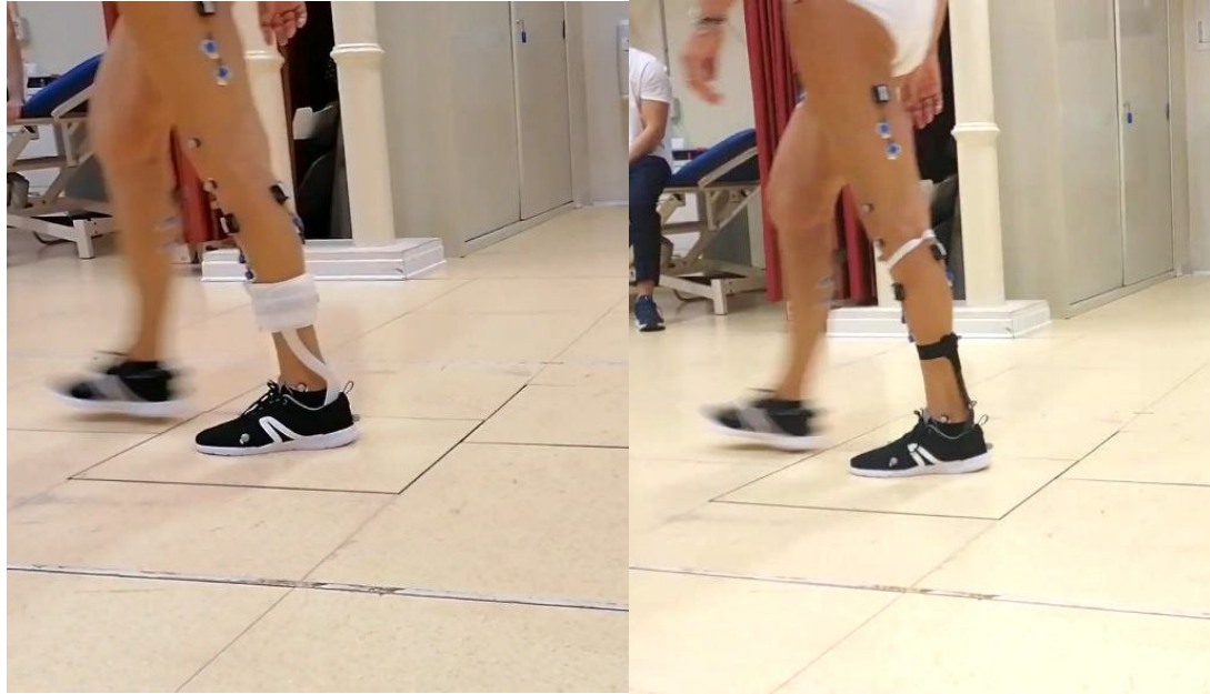
Figure 36: Gait analysis walking trials by a patient wearing a Codivilla spring (left) and the custom AFO (right) on the left foot. On the floor the two “hidden” Kistler force platforms are visible.
