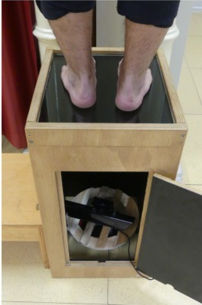
Figure 21: The Kinect-based 3D foot scanner.
