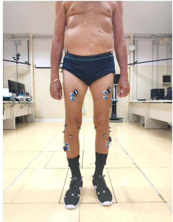
Figure 32: The body markers' positions according to the IOR gait kinematic protocol: on the foot they are positioned on the first (FM), second (SM) and fifth (VM) metatarsal head and on the calcaneus (CA), while LM and MM track the position of the lateral and medial malleolus of the ankle respectively.
