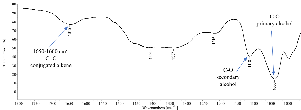
Figure 91: FTIR of hydroglycolysis products obtained using glycerol. Range 1800-1000 \text{cm}^{-1}
