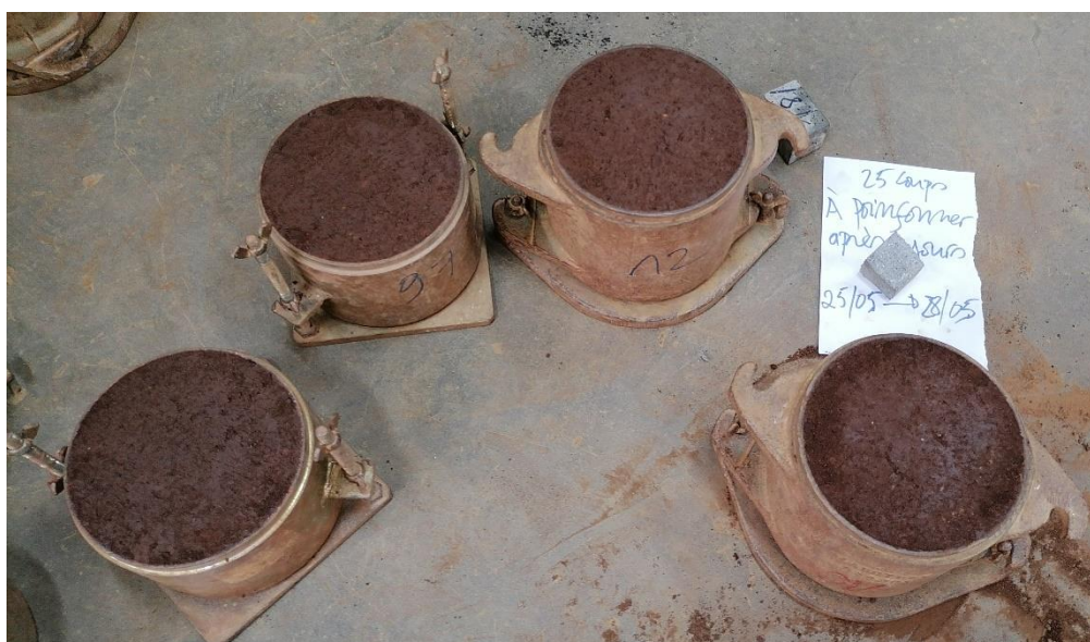
Figure 4. 10. CBR samples of AggreBind treated soil
