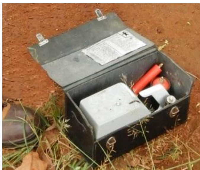
Figure 6: Piezometric measurement with floating (orange) and sinking (grey) heads
