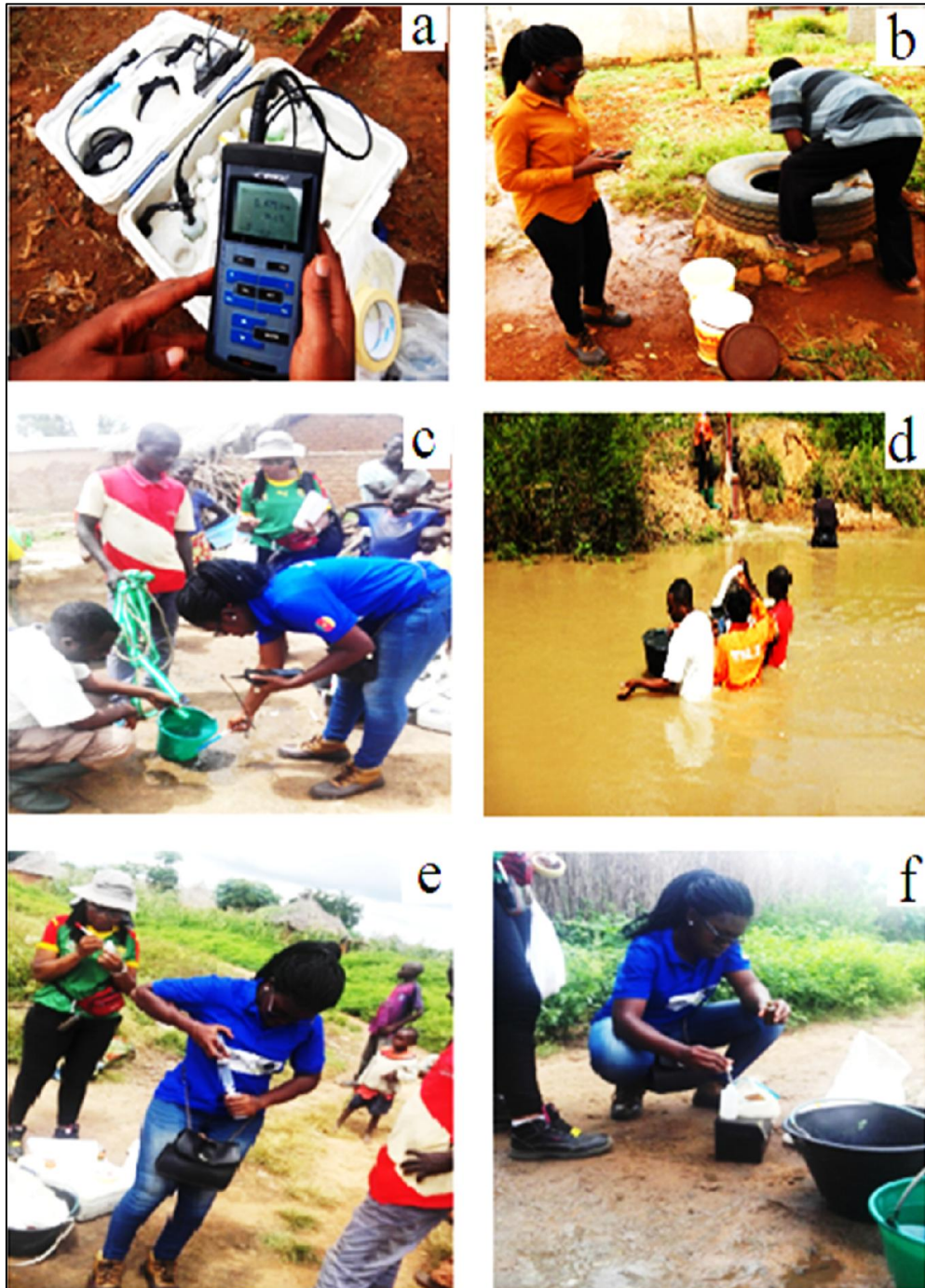
Figure 4: Important steps of water sampling: calibration (a), geo-localisation (b), rinsing of the electrodes with water sample (c), measurement of in-situ parameters (d), filtration (e), acidification (f)
