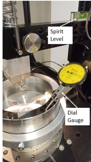
Figure 5. 26: dial gauge and spirit level to ensure vertical alignment.
