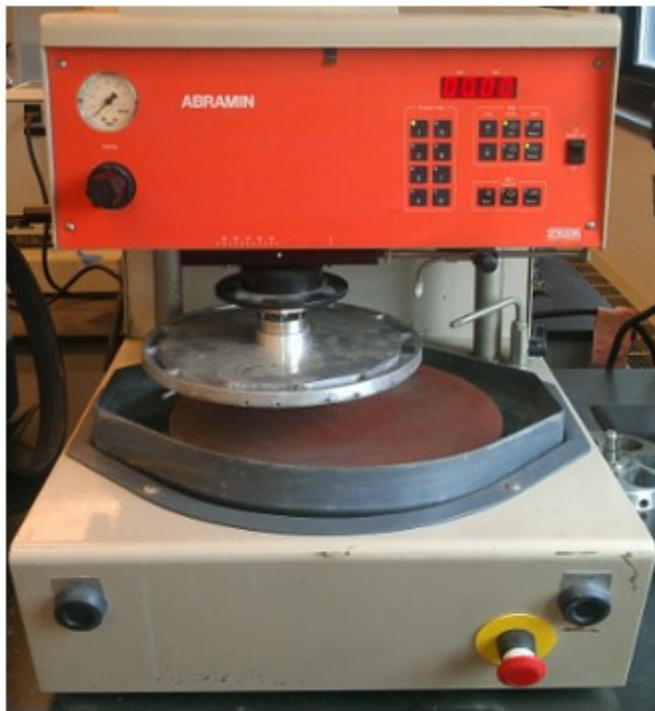
Figure 5. 14 Abramin controlled machine, source: https://engineering.case.edu/research/labs/materials-science-metallography-lab/struers-abramin (left), sample holder before polishing (right)
