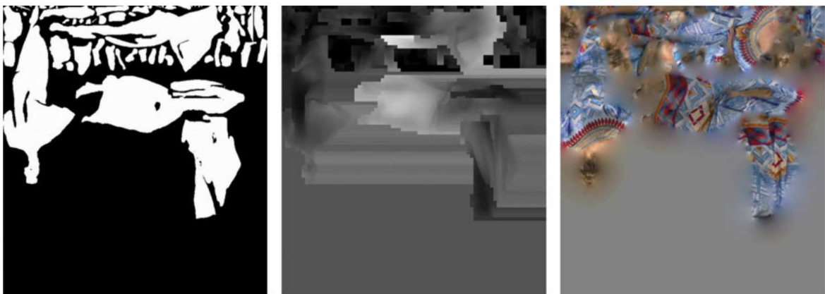
Figure 2.7: Example of packed patches, respectively: Occupancy map, Geometry map and Texture map [4]
