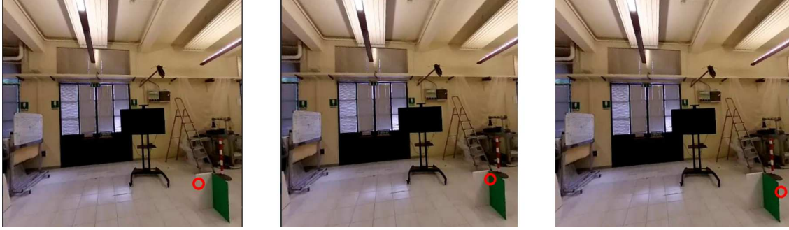
Figure 4.4: Sample of transforming point from the robot plane to image plane to evaluate H matrix.
