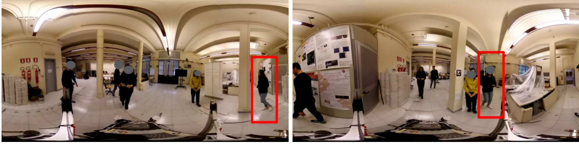
Figure 4.7: Switch ID during tracking. a) before the person misses in the frame. b) after remerging the missed person.
