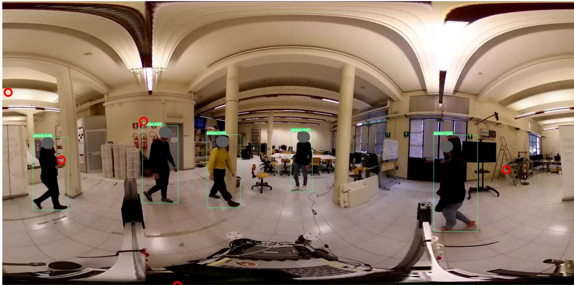
Figure 3.7: Result of transform points from the robot plane to the image plane by applying the procedure of computing H matrix on the panoramic image.
