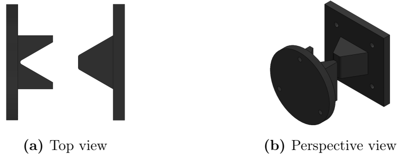
Figure 39: CAD model of the V-shaped probe-drogue design
