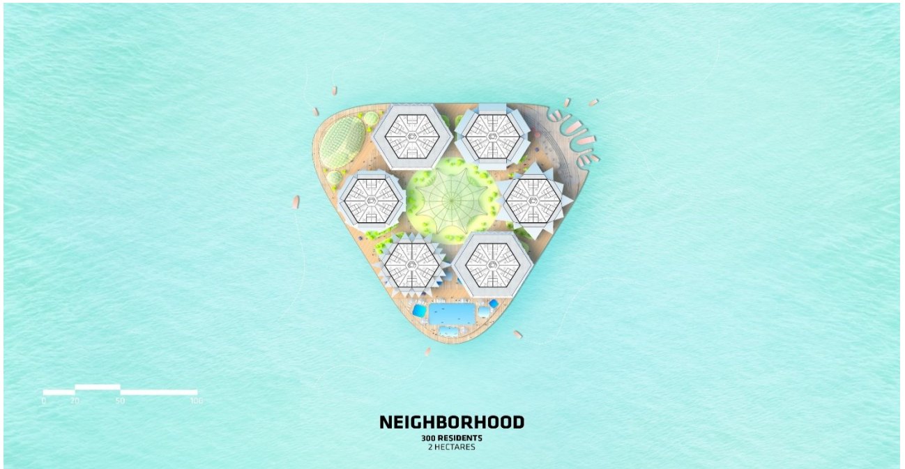
FIGURE 30: Design of a single neighborhood platform unit as envisioned in the OCEANIX City project (OCEANIX/BIG-Bjarke Ingels Group).
