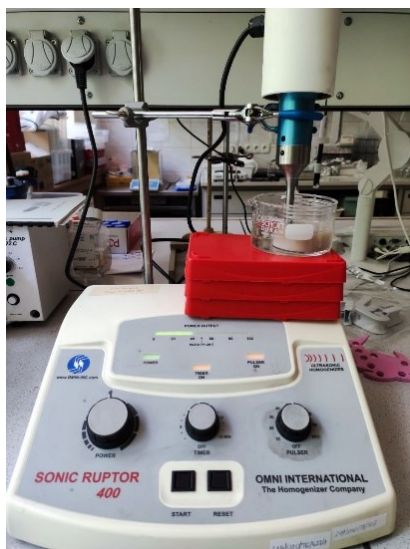
Figure 19: Sonication homogenization procedure Figure 20: Final sample product: Left RT-DND-LN, Right RT-DND
