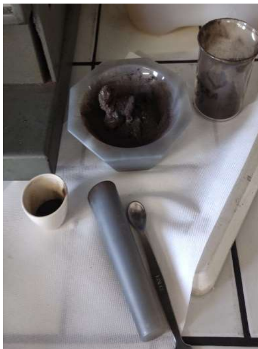
Figure 11: Perovskite after the dehydration step
