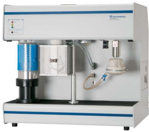
Figure 20: TPR tool used in laboratory
