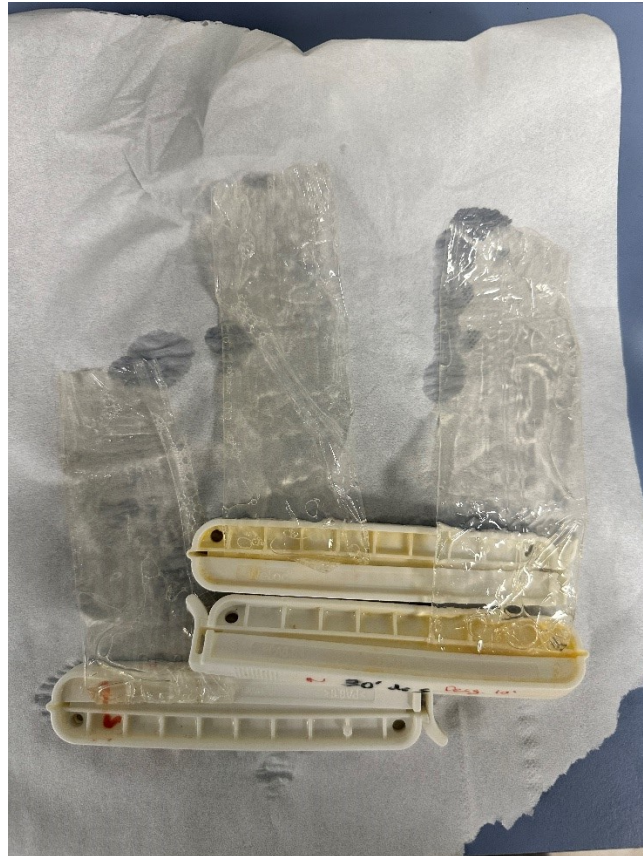
Figure 2.2 – Cut off membranes after dialysis and reverse dialysis.
