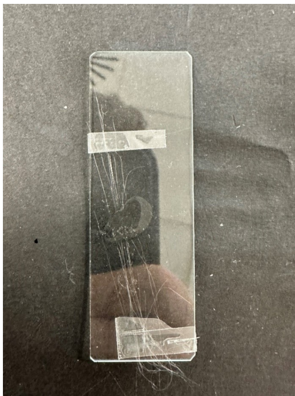
Figure 4.2 – Silk fibroin fibers aligned in a laboratory glass. A drop of water is made to fall on the fibers. Although is difficult to see, from a closer look fibers are still visible even in contact with water. This assesses the insoluble state of fibroin fibers.
