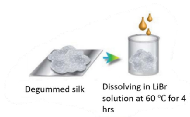
Figure 2.1 – Simple representation to transform degummed silk into a fibroin-LiBr solution.
