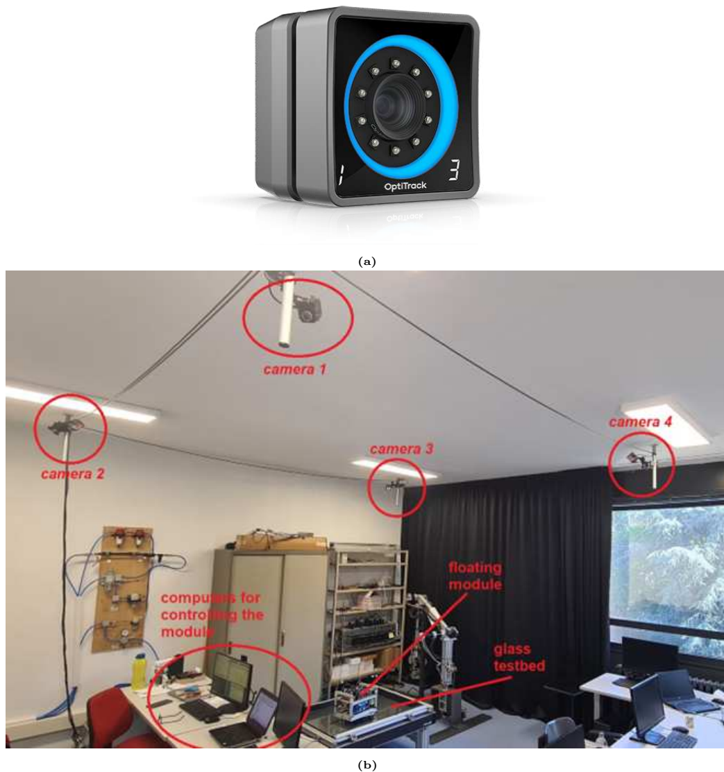
Figure 4.19: (a) Motion capture camera, model Prime x 13 made by OptiTrack , and (b) test setup for the inertia estimation of the module.
