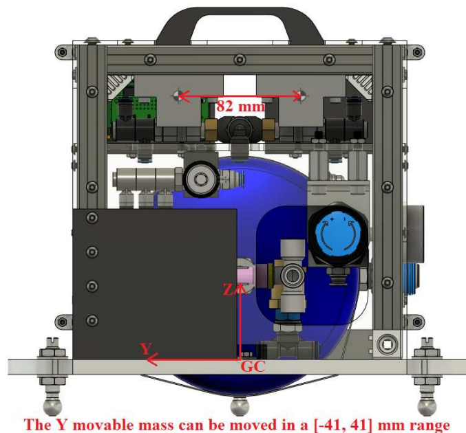
Figure 3.34: Extreme positions of the Y movable mass.
