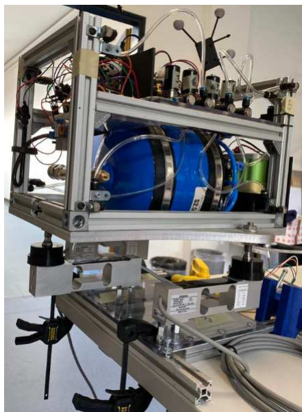
Figure 4.6: Assembled module on the anchored load cells platform.
