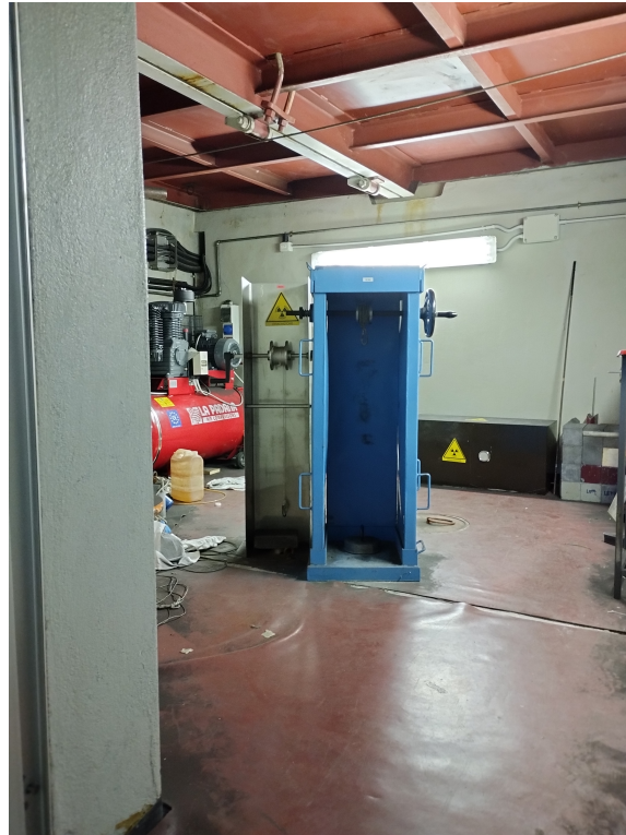
Figure 5.5: Picture of the pulley used to place the Petri dishes containing the cells in proximity of the cobalt source.
