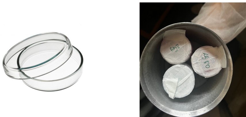
Figure 5.4: On the left, of the Petri dishes used for the experiment [47]. On the right, picture of the Petri dishes labelled with the dose of irradiation; the ones unlabelled are not irradiated and used as "control" samples.
