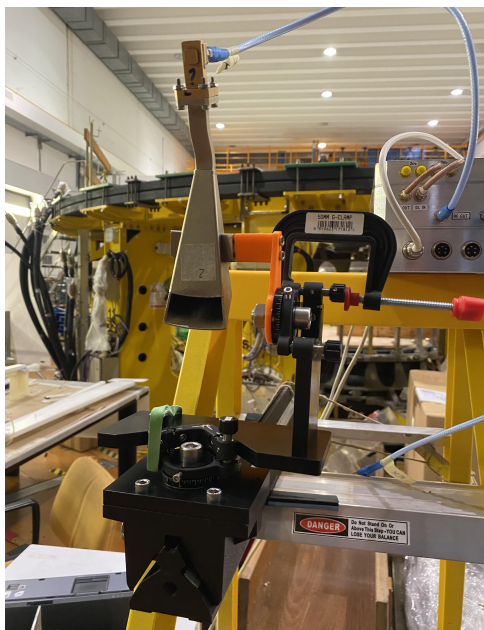
Figure 4.4: Picture(left) and CAD model(right) of the hoghorn antenna mounted on its support
