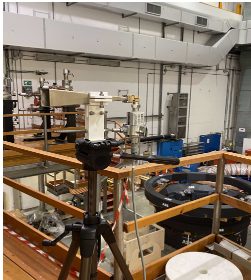
Figure 4.2: Receiving antenna mounted on its tripod
