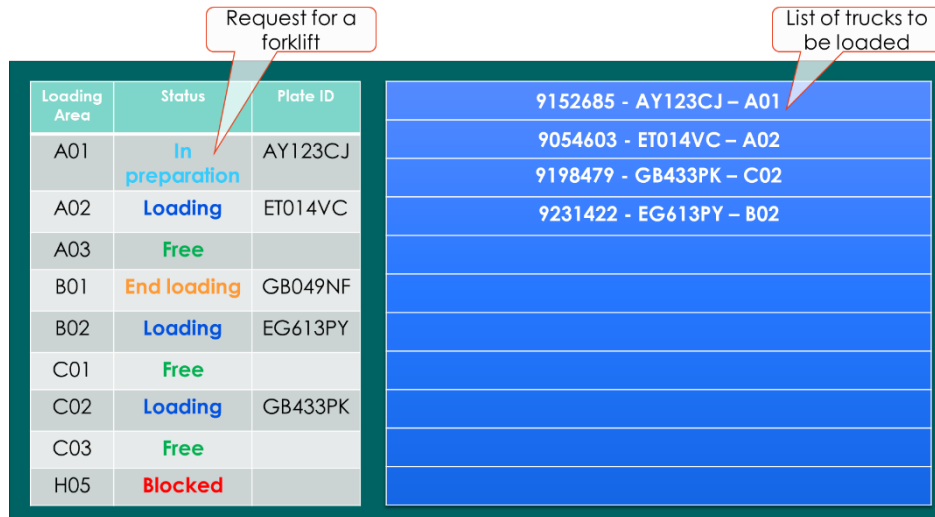
Figure 3.7 New visualization in the Pallet Tracking System for the shipping operations [14]
