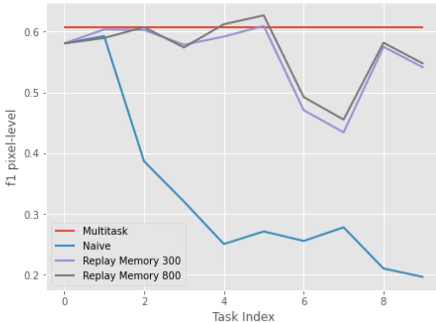
Figure 5.3: Comparison of pixel-level f_1 metric trends as new tasks are added across various strategies.
