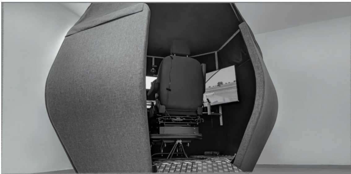
Figure 3 Dynamic driving simulator (Nervtech™, Ljubljana, Slovenia) located at the Neuroergonomics & Operator Performance Lab (CIMCYC, Universidad de Granada, Spain).
