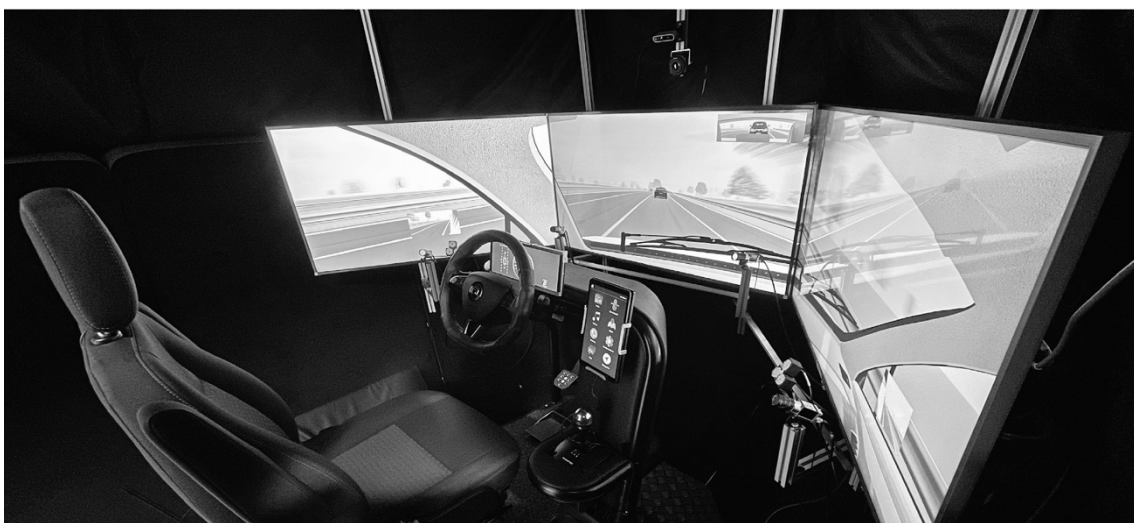
Figure 4 Inside of the dynamic driving simulator (Nervtech™, Ljubljana, Slovenia) located at the Neuroergonomics & Operator Performance Lab (CIMCYC, Universidad de Granada, Spain). Three 49"
