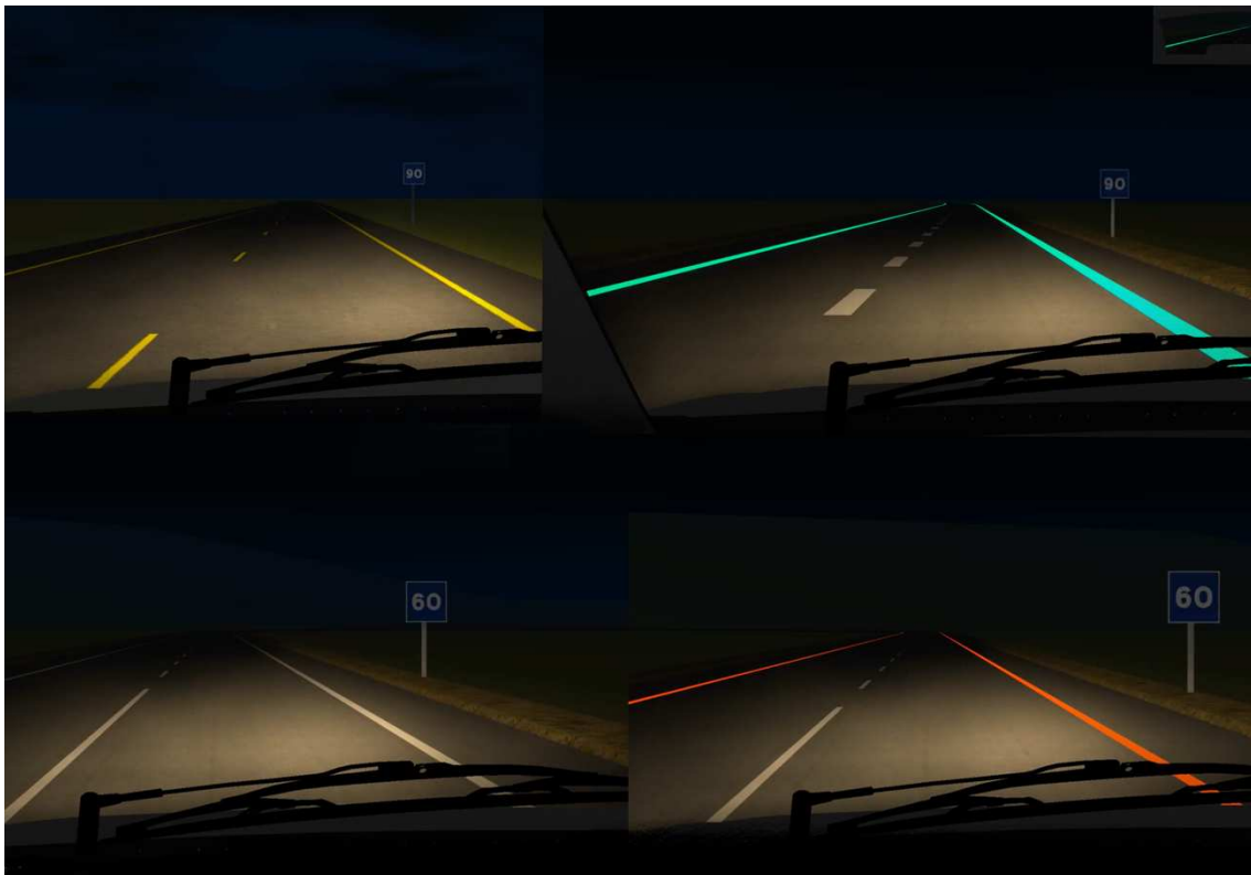
Figure 5 Central screen of the simulator and recommended speed limits (90 km/h or 60km/h) placed at the beginning of each of the curves displayed for the video-based perception task. In yellow: the training video; in green, red, and unlit: the experimental curves.
