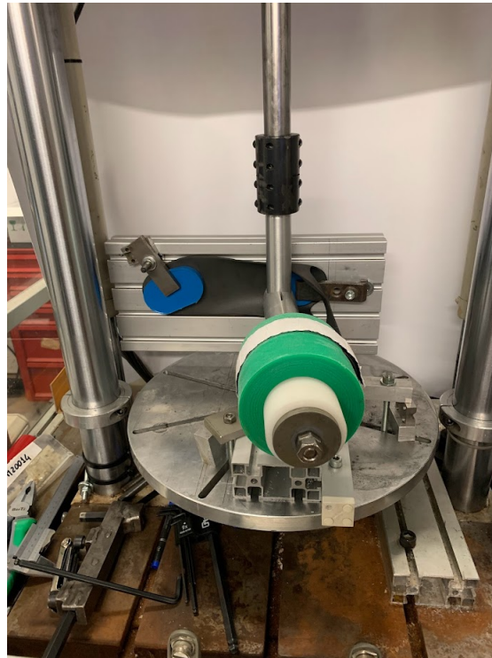
Figure 2.6: The new setup to determine AFO stiffness with an AFO positioned.
