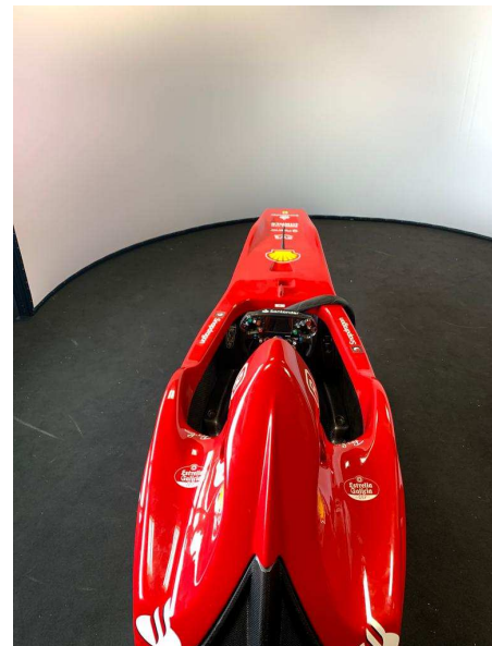
Fig. 39; Fig. 40 – Replica of the “Maranello” set up. The difference between this and the one used to collect the data consist in the screen. Here a 180-degree curved screen is present. The original set up included 3 flat screens.
