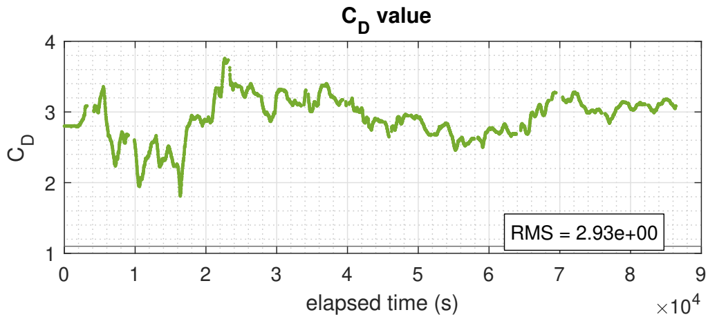
Figure 7.3.4: C_D parameter value over time during EKF estimation.
