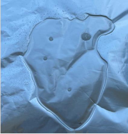
Figure 8a. 10 % w/w PVA sprayed on a collector Figure 8b. 10% w/w PHB dissolved in Cyrene sprayed on collector
