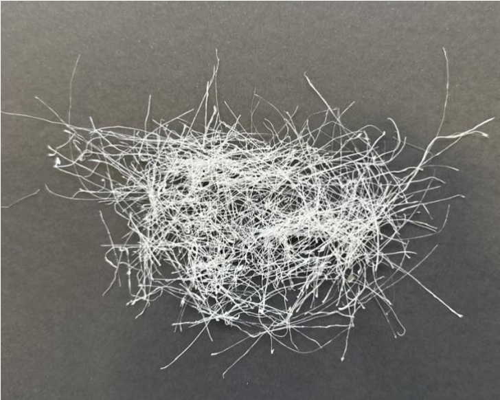
Figure 9. Image of 2 % w/w chitosan fibers
