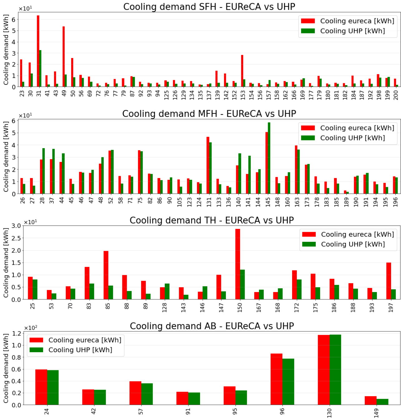
Figure 3. 18: Cooling consumption per building category – residential sector
