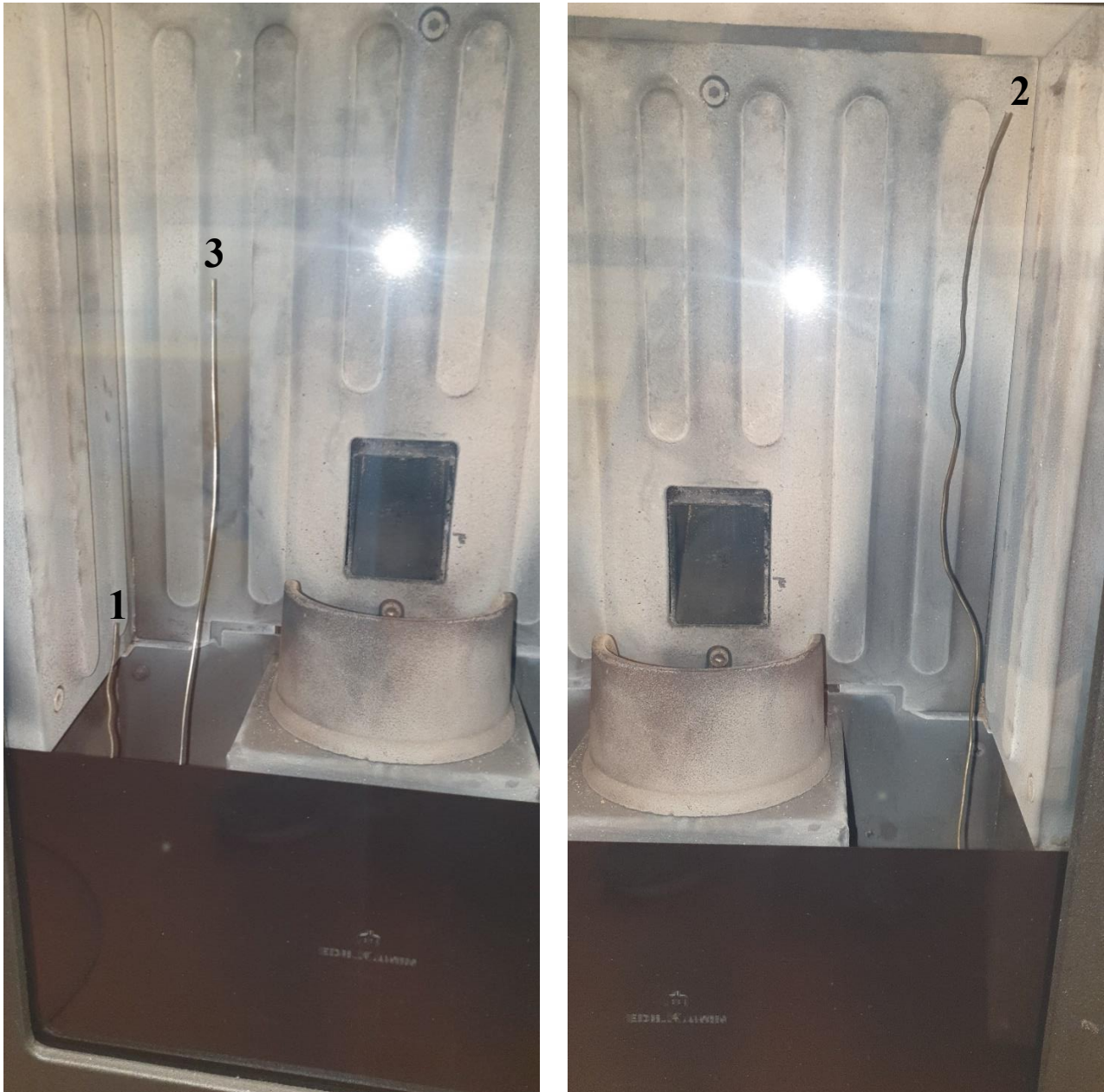
Fig. 3.14: thermocouples placed for Temperature Test 2
