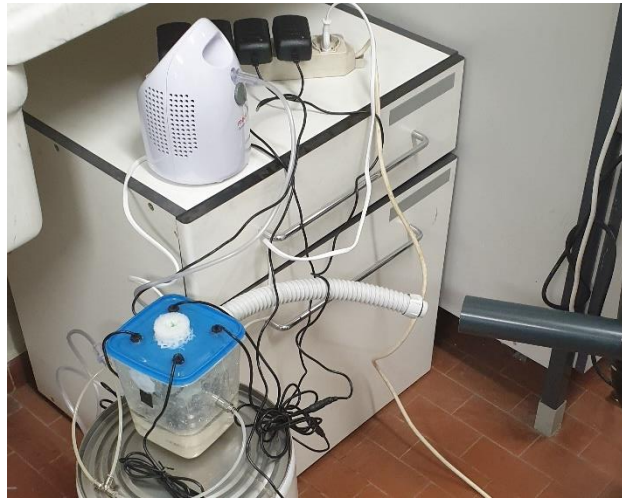
Fig. 3.49: vapor test experimental: nebulizer, plastic box and flexible tube
