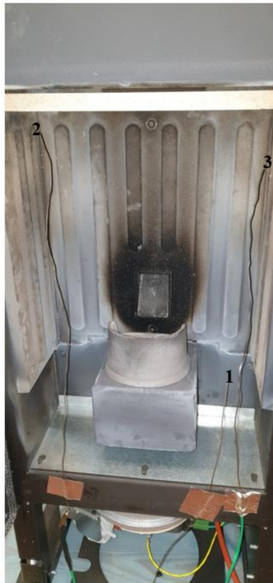
Fig. 3.16: thermocouples placed for Temperature Test 3
