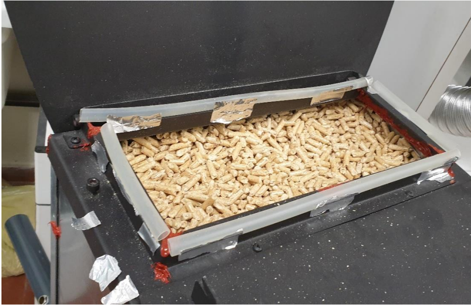
Fig. 3.50: tank cover sealing for 20 kg load tests
