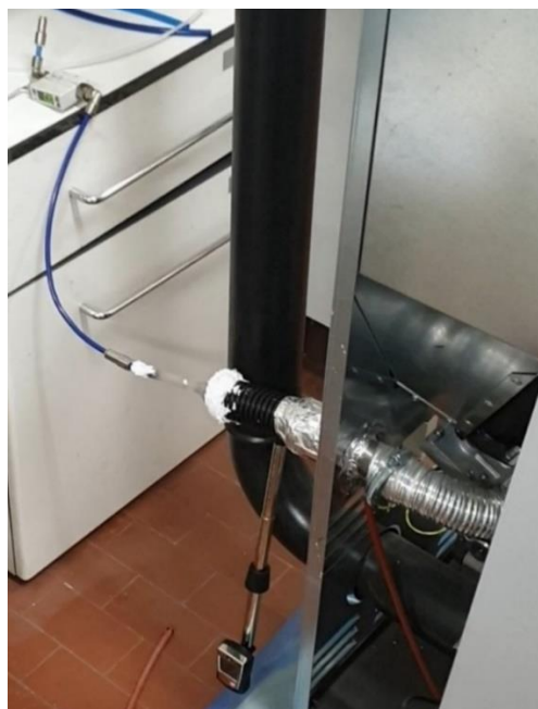
Fig. 3.45: inlet velocity experimental line: portable anemometer, rigid tube and flowmeter
