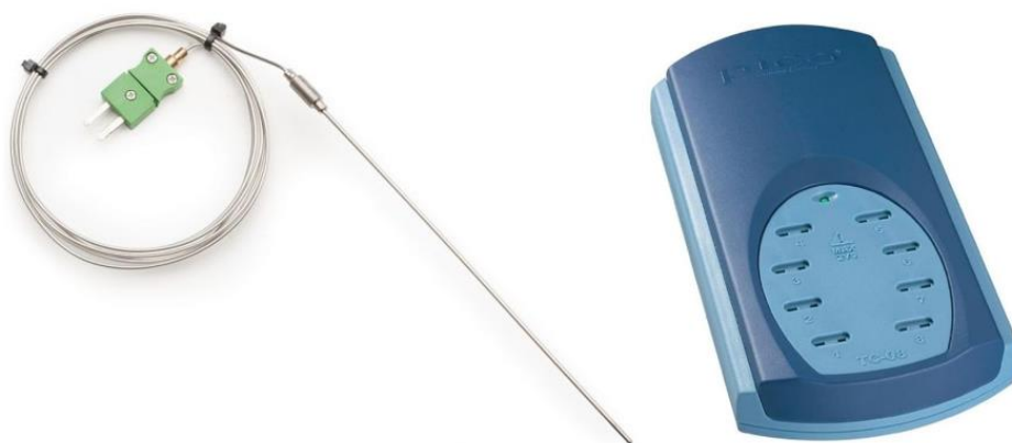
Figure 2.8: K-type thermocouple (1) and Picolog data logger (2)
