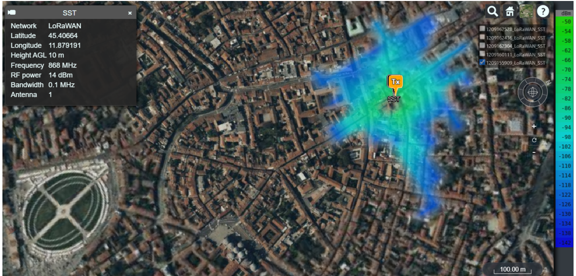
Figure 4.5: Coverage Map with Longley-Rice model SF7
