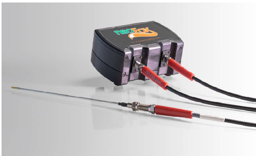
Figura 4.9: Neofox Oxygen probe developed by Ocean Insight.
