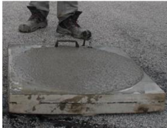
Figure 1.2. flow test (structure course, 2015)
