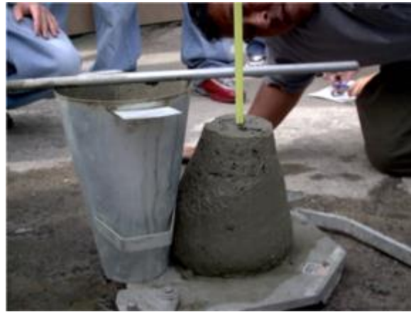
Figure 1.1. slump test (structure courses, 2015)
