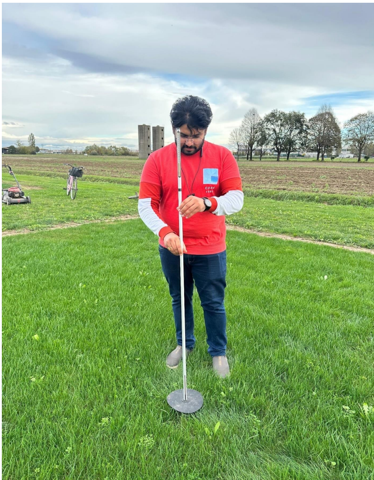
Fig1. Measurement of the height of the turfgrass before mowing using grass plate meter.
